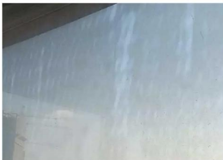
● 自然光下应力斑严重，目视清晰可见 Serious stress mark in natural light, clearly visible to the eye
